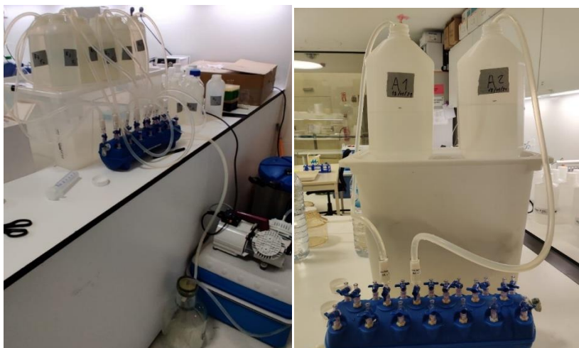
Figure 7: The filtration system used for filtration, where the vacuum pump pulls the water contained in the bottles, through the Sterivex filters, concentrating the biomass present in the environment.
